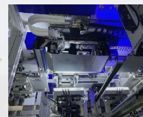
4.软(sensor)对硬(盖板)贴合 Soft to hard Laminating
